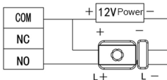
Figure 3-3 Magnetic lock cable connection
