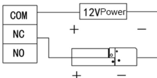
Figure 3-5 Door contact and exit button cable connection
