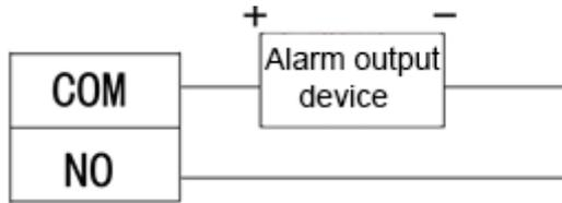
Figure 3-7 Peripheral alarm output device cable connection (2)
